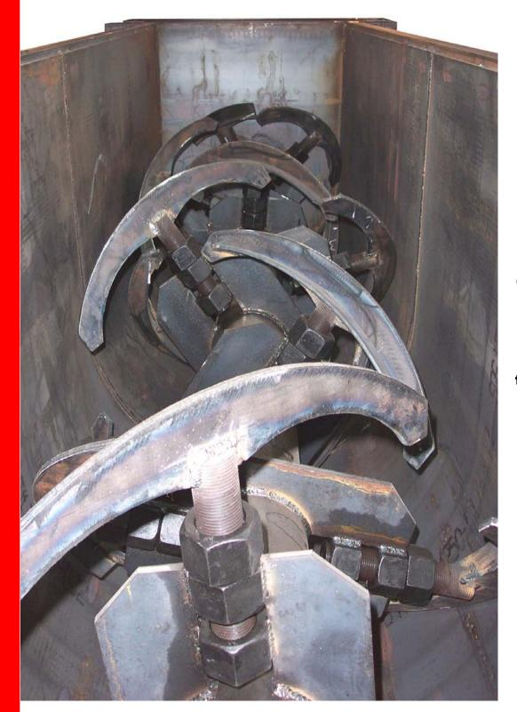
**Our continuous** mixers are built with **BOTH** the forward and the reverse paddles adjustable. In addition, the discharge gate can be adjusted to control the depth of material in the mixer. Combining these features with a variable frequency drive (VFD - supplied by others), **OPERATOR WILL** HAVE FULL **CONTROL OF RETENTION TIME.**
