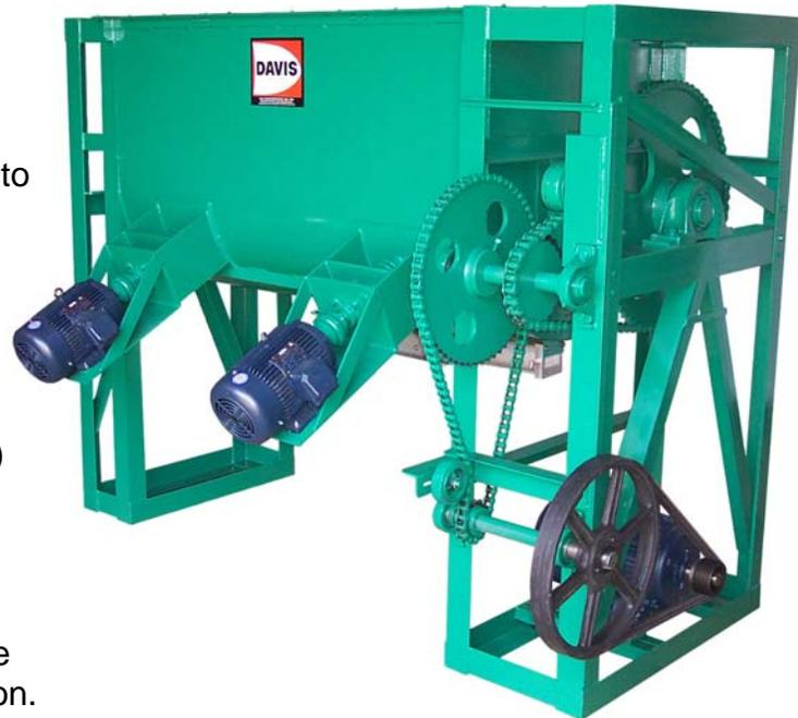
We offer various drive options to suit each customer's application and budget. Triple speed reduction is required to reach the appropriate final speed recommended by Davis Manufacturing.
