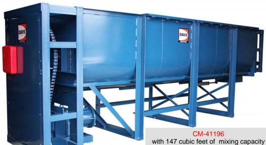
with 147 cubic feet of mixing capacity high legs, foot mounted gear box with 40 H.P. and air cylinder on outlet. Shown with protective guards removed.
