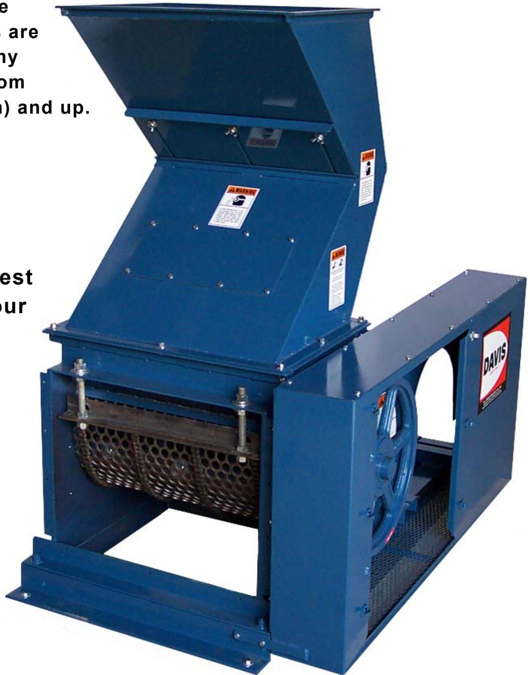
The Rotary Knife Cutter has full access panels on both sides so that the screen can be easily changed in just a few minutes.
